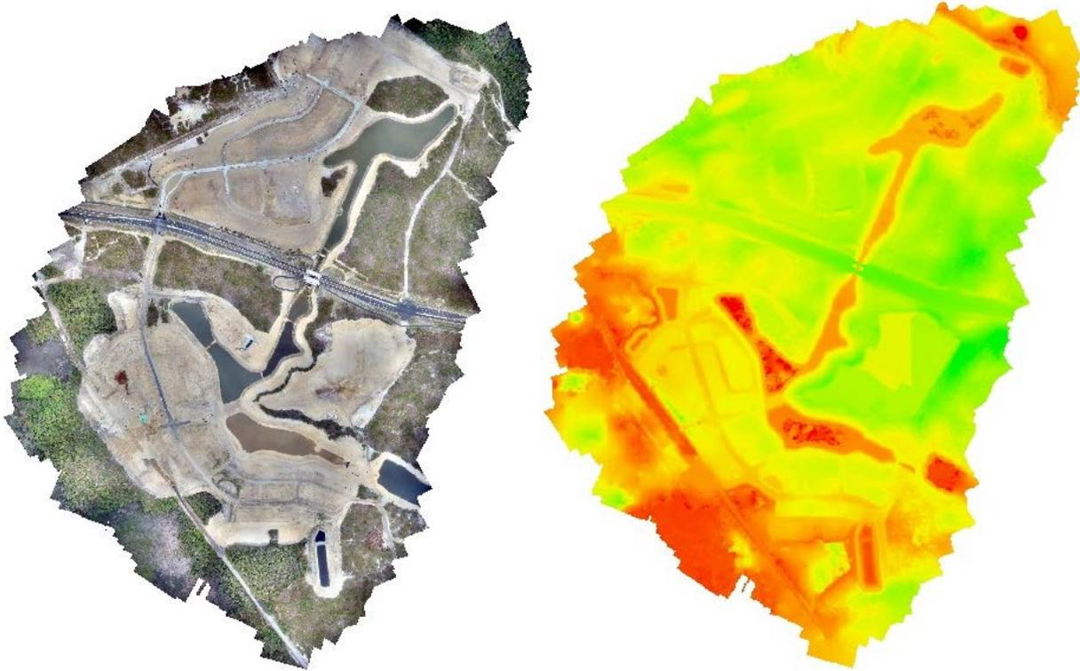
*Figure 4: Construction Site Orthophoto & Digital Surface Model*
