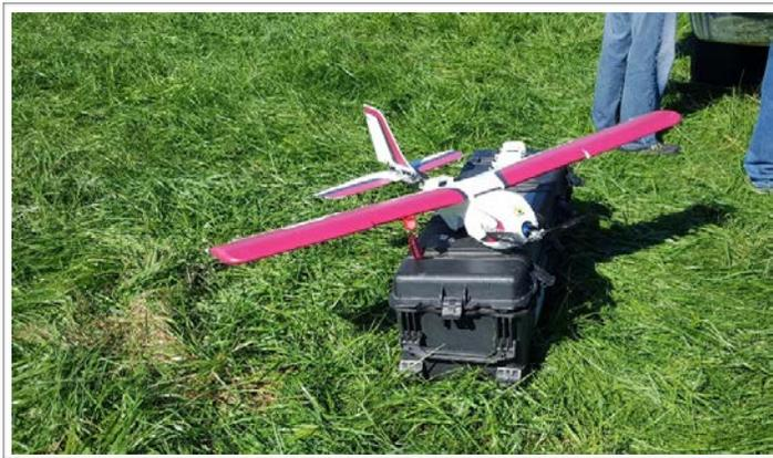
*Figure 24: Precision Hawk Lancaster Aircraft Pre-flight*
