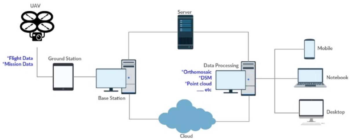
Figure 34: Example UAS Data Architecture
